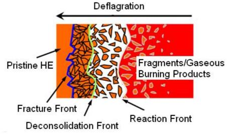
Figure #5 - Damaged reaction zone burning
